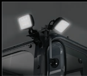
Forward and Left-Facing LED Light (Cab)
