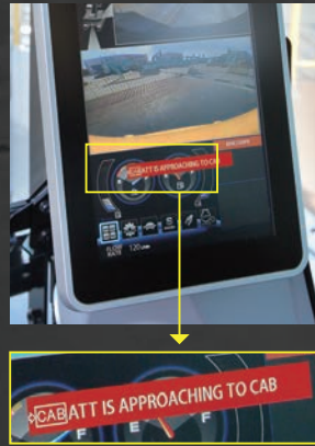
Cab interference warning
