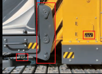
Easy lubrication for elevator cab The grease nipples for lubricating the elevator cab are gathered in one place.
