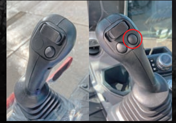
Proportional slides on the joysticks with power boost switch (right control lever)
