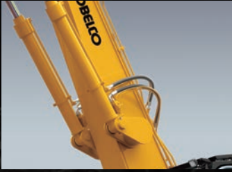
Scrap loader straight boom (1-Pin)
