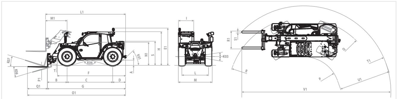
Figure: 180201-1: Dimensions with standard wheels
