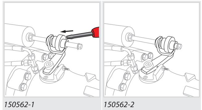
The parking brake must be disengaged directly on the axle to allow the vehicle to be towed.
