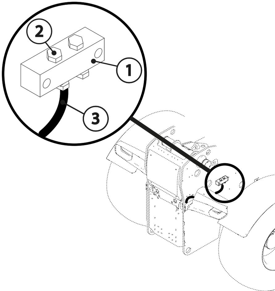
1 - In case of malfunctioning and/or emergency, connect an external pump to the port "2" on pipe "3" in order to lift the boom.
