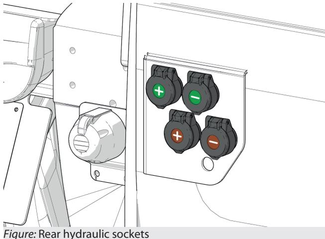
Figure: Rear hydraulic sockets
