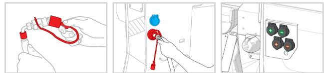
Cap and mark on the hydraulic sockets.
