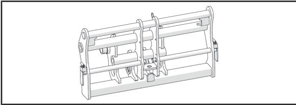
The attachment holding plate is the interface between the vehicle (telehandler) and the interchangeable equipment. The attachment holding plate is placed at the end of the telescopic boom and is used for the quick and safe installation of the interchangeable equipment at the vehicle base.
