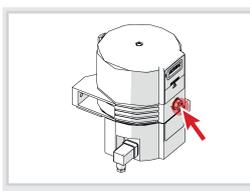
Automatic lubricator system filling
