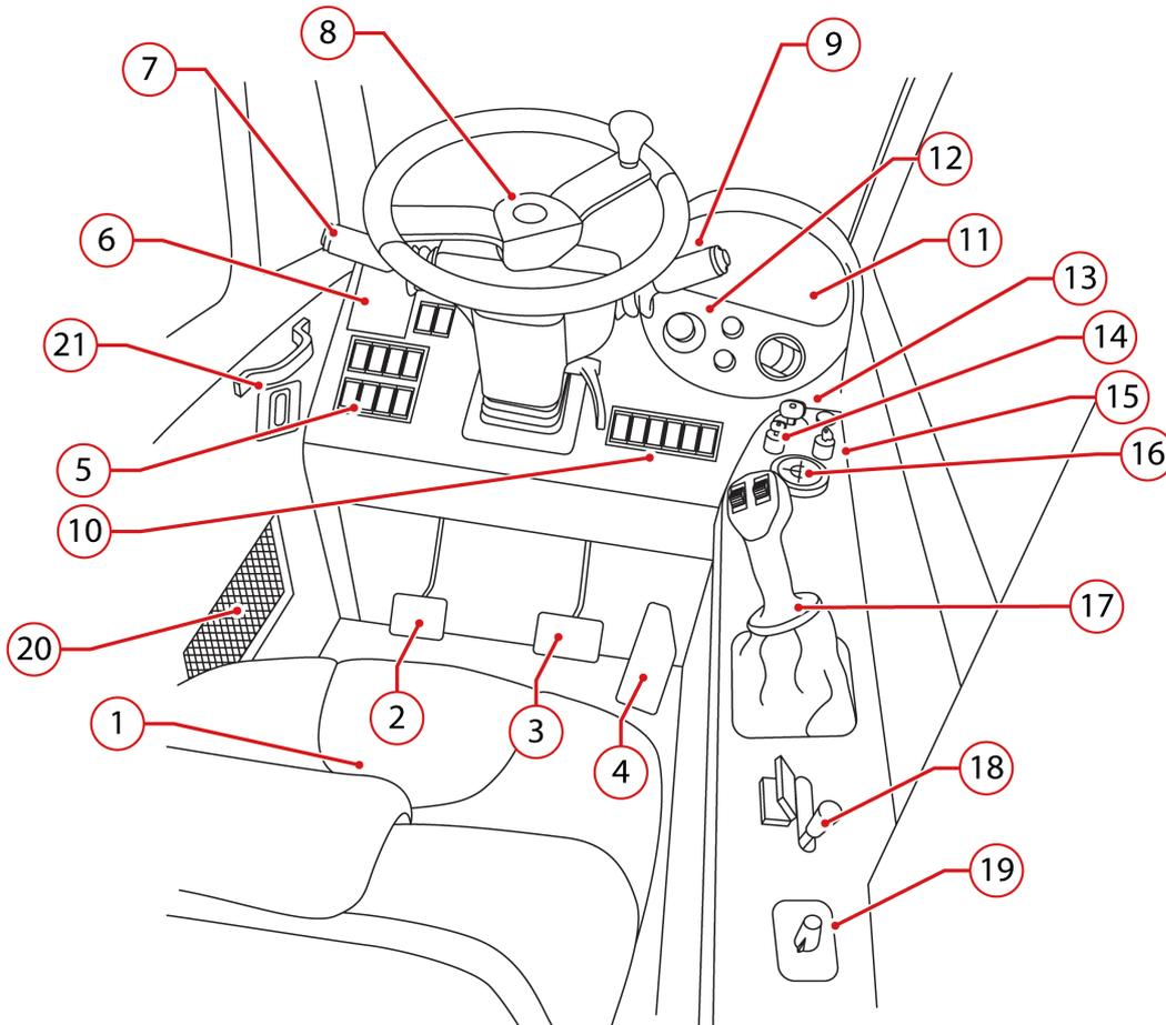
Figure: 150989: Components inside the cab
