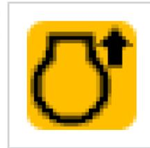
If the user does not increase the engine rpm, the vehicle will automatically increase the rpm to 1200 or 2000 according to the need.
