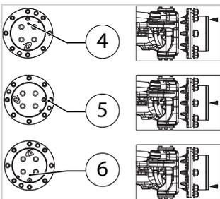
To fill the oil, turn the crown and position hole "4" upwards.
