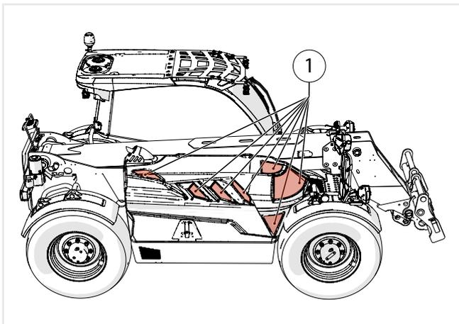
Check that the air recirculation networks and grids "1" are clean and free from dirt: for cleaning use a jet of air at low pressure from the inside to the outside of the vehicle.
