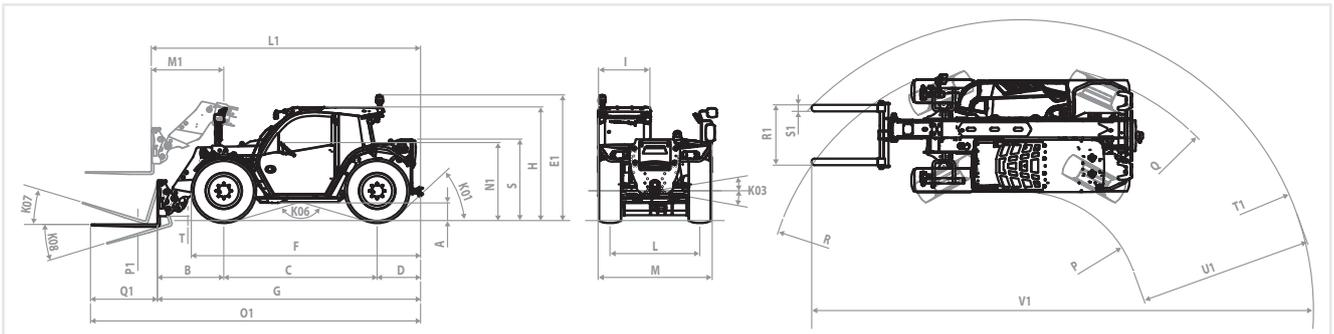
Figure: 180201-1: Dimensions with standard wheels
