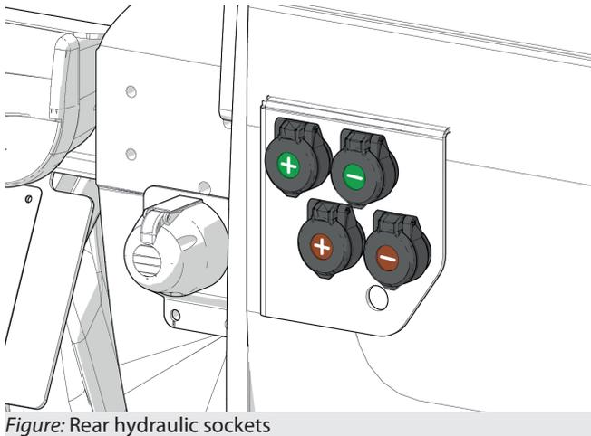
Figure: Rear hydraulic sockets
