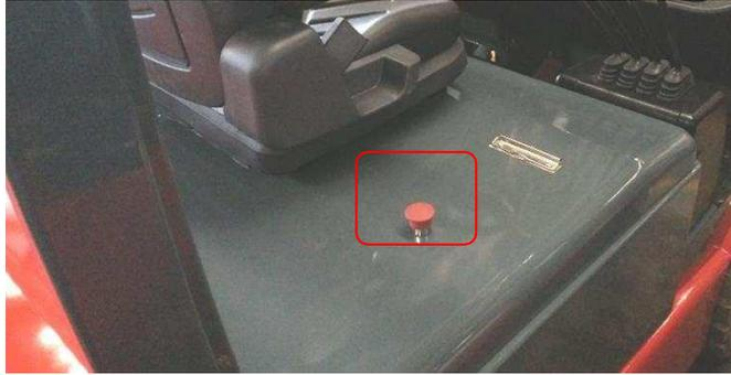
Figure 4-7 Emergency power off switch
