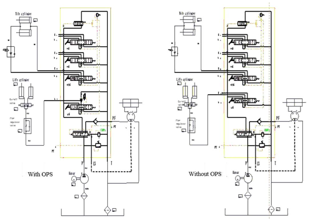
Fig. 5-12 Schematic diagram of hydraulic system
