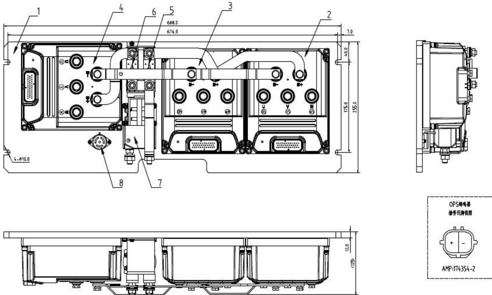
1. Bottom plate 2. Driven AC controller 3. Drive AC controller
