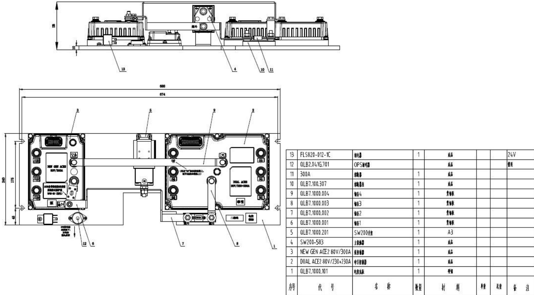
1. Electric control plate 2. Drive controller 3. Pump controller 4. Main contactor 5. SW200 bracket 6. Copper bar 1
