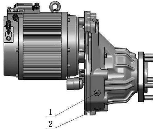
Fig.1-3 Position of each oil hole
