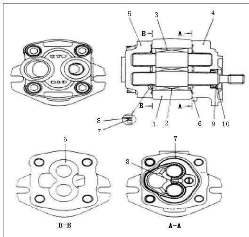
Figure 5-2 Gear pump structure outline diagram
