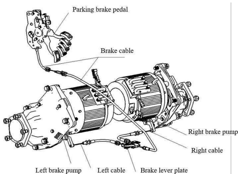
Fig. 2-4 Parking Brake Action Schematic
