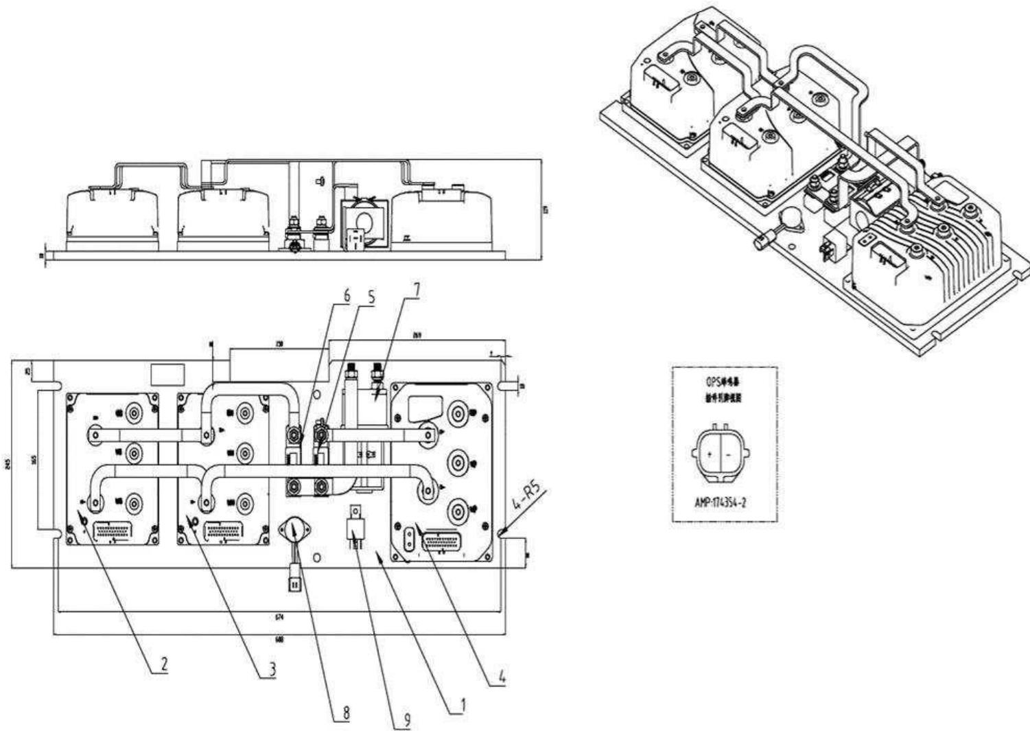
1. Bottom plate 2. Driven AC controller 3. Drive AC controller 4. Pump AC controller
