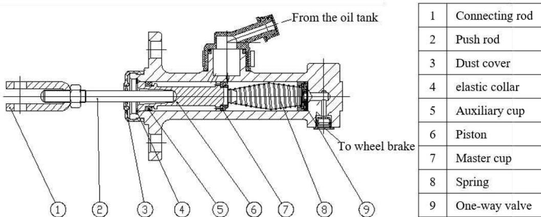
Fig.2-3 Brake master pump
