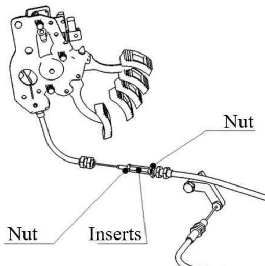
Figure 2-7 Parking Brake Cable Adjustment
