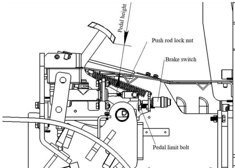
Fig.2-2 Brake pedal adjustment
