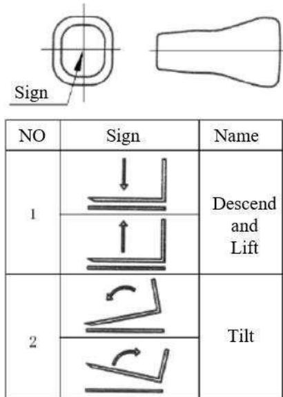
Fig. 5-5 Multi-way valve control handle identification
