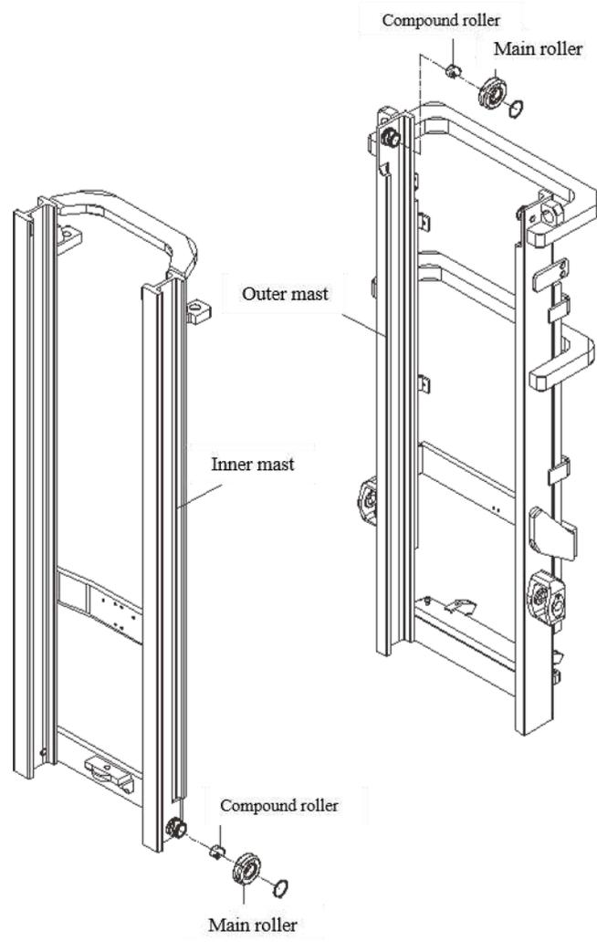
Fig. 6-7 Inner and outer mast
