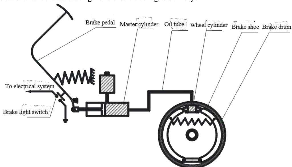
Fig. 2-1 Principle diagram of service brake
