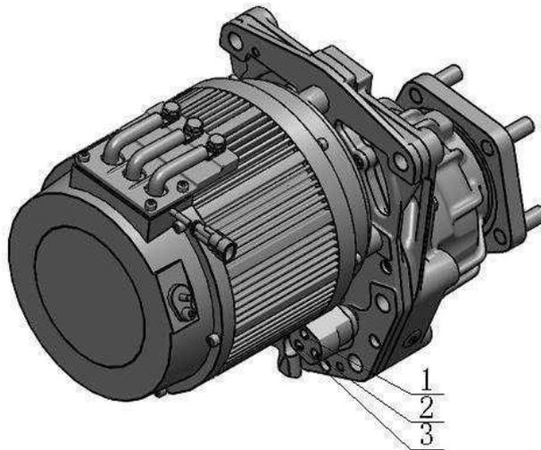
Fig.1-4 Position of brake oil port
