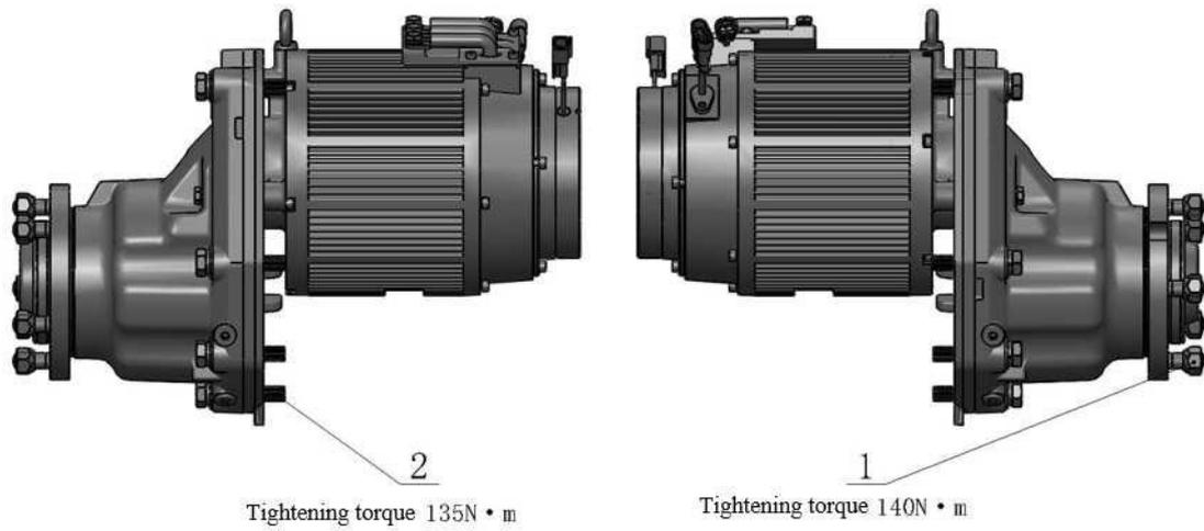
Fig.1-6 The drive axle and external connection
