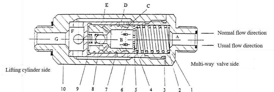
Fig.5-10 The speed limit valve
