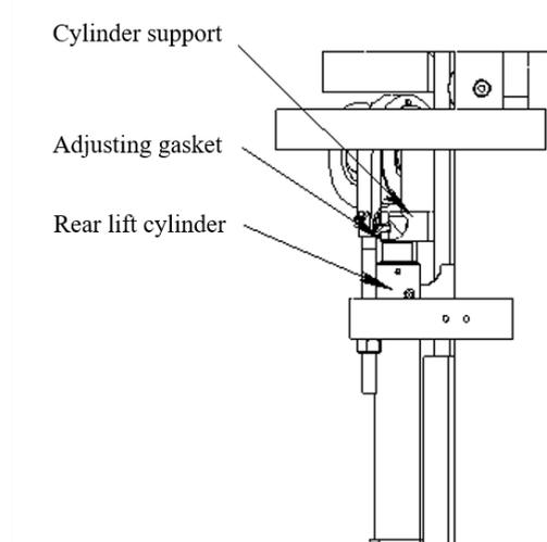
Fig. 6-17 Adjust rear lifting cylinder synchronously
