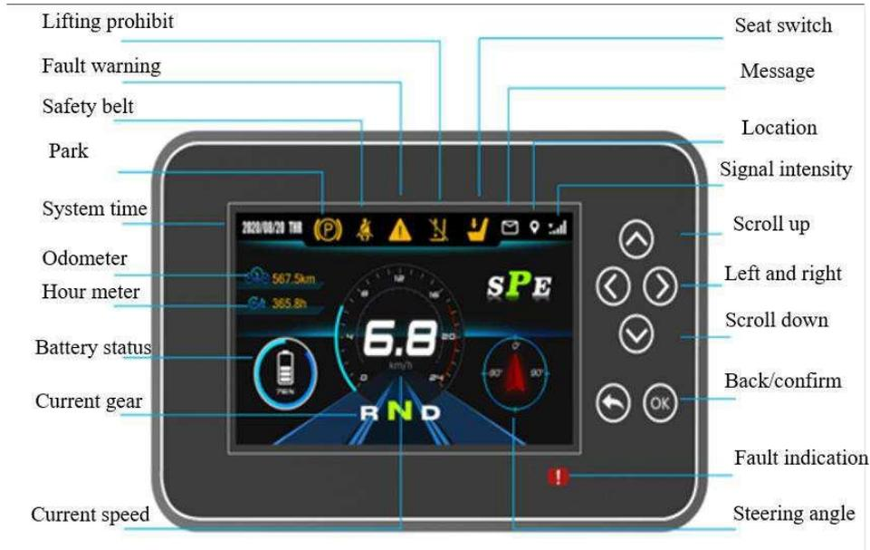
Fig. 4-2 Panel layout of technology system
