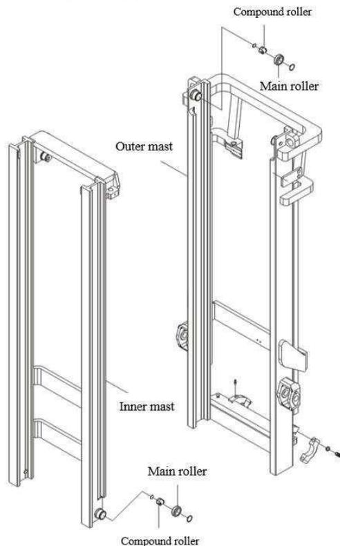
Fig.6-1 Inner and outer mast
