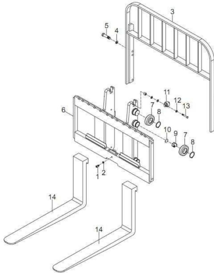
1. Limit screw 2. Washer 3. Load-backrest 4. Washer 5. Bolt 6. Fork carrier
