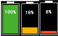
3401T-5002 The battery icon on the main interface of the table would be displayed in different colors according to the battery quantity. The battery quantity range is 0~100%. The specific meanings of battery icons are as follows:
