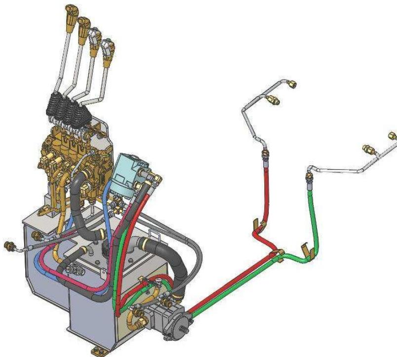
Fig. 5-13 Hydraulic Piping Diagram
