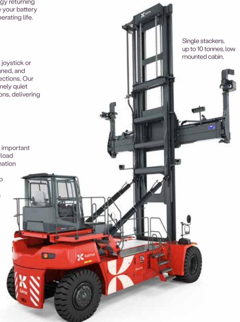
Single stackers, up to 10 tonnes, low mounted cabin.
