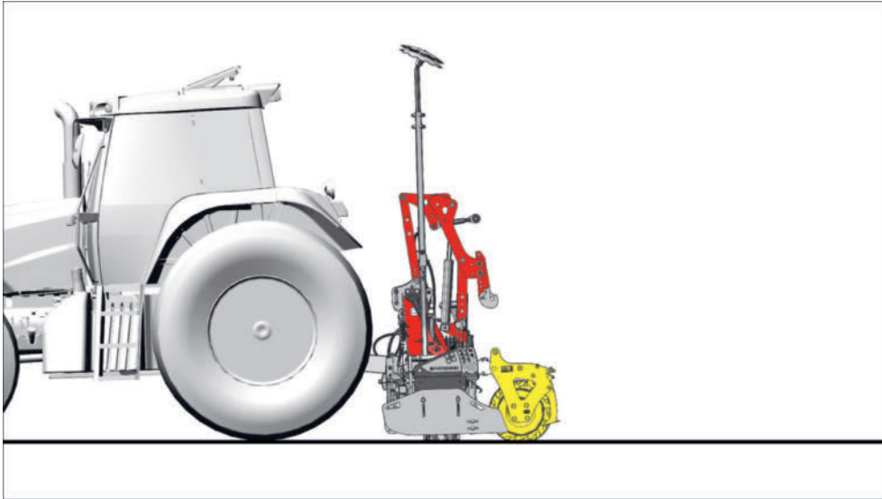
Fig.: Working position; hydrolift in road transport position / headland position
