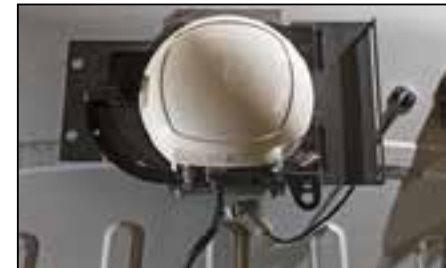
The AUTO-GUIDE 3000 TopDock contains a 72-channel Global Navigation Satellite System (GNSS) satellite receiver along with high-end inertials that maintain accuracy in side-hill operations. Adding the Decimeter Snap-In Module for two to four inch accuracy and adding a second Centimeter Snap-In Module for less than one inch accuracy enables the system to operate at the levels the customer requires for their operation. With the Centimeter Snap-In Module, the owner can choose between a Mobile Base Station or the use of an Internet Correction Source, such as a Continually Operating Reference Station (CORS).
