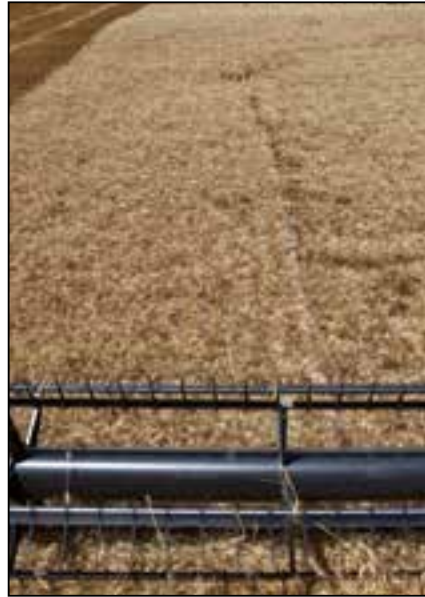
Using cutting edge Global Navigation Satellite System technology, Gleaner's new AUTO-GUIDE 3000 system will steer the combine through the field. This helps the operator maintain a full cut on the header and improves the efficiency of the entire harvest operation and reduces operator fatigue.
