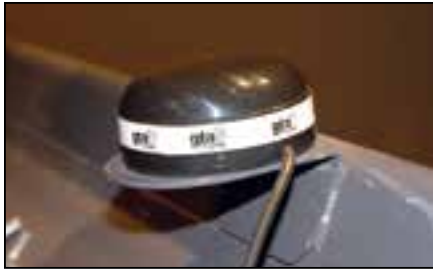
The DGPS antenna for the Fieldstar® II yield-monitoring system receives its information from the WAAS Satellite System to pinpoint the field location.
