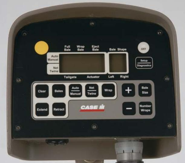
The Electronic Auto-Controlled Twine/Mesh Wrap System allows you to control operations right from your tractor cab. With a few simple keystrokes, you can adjust bale size, change tying patterns, monitor your bale count and engage diagnostic functions.
