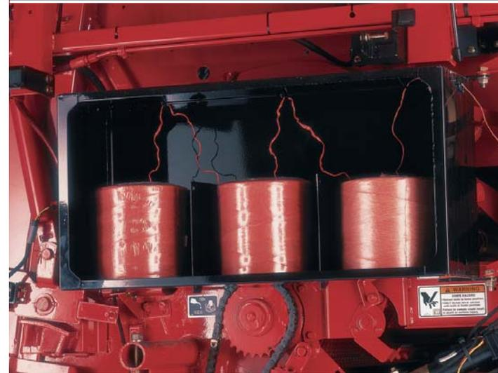
The twine boxes, mounted on each side of the baler, offer plenty of storage. All twine/mesh balers hold six balls of twine and two rolls of mesh. Optional twine boxes are available to hold up to maximum of 12 balls of twine.
