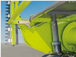
Adjustable crop press bars, optionally with hydraulic operation.
