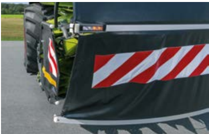
Side and front protection clearly visible with warning stickers. The LED lighting is fully integrated.
