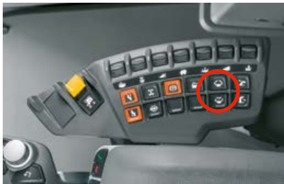
One switch for the entire folding process.
