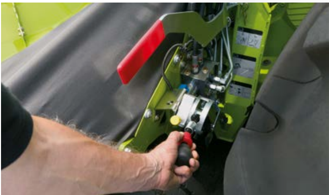
Three-stage speed adjustment of intake drums for optimal crop flow.
