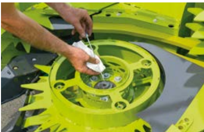
Dipstick to check oil level.
