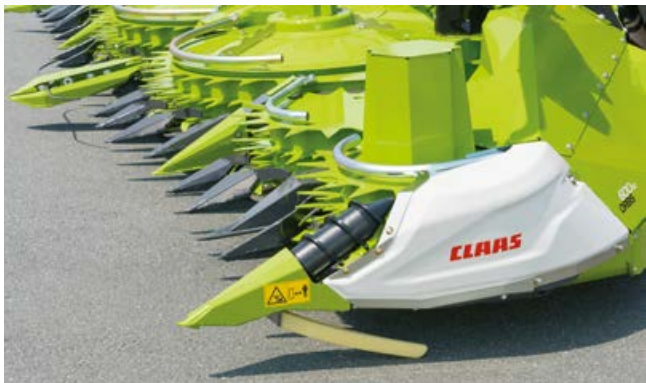
If required, the laid maize augers are driven hydraulically.
