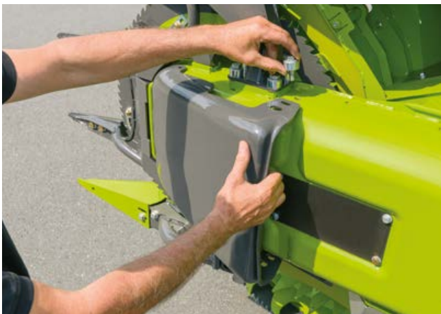
Skids with two height settings.
