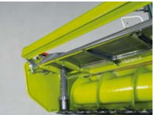
Roller crop press for a very even crop feed.
