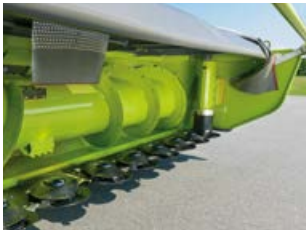
DIRECT DISC 600 / 500 with large intake auger.
