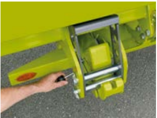
With the front attachment locked in place, it is possible to travel safely at up to 40 km/h.
