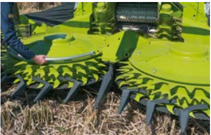
Removal of cob retainers increases crop flow performance.
