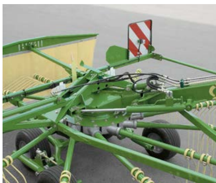
Shifting the rear rotors left/right Operators can quickly shift the rear rotor to the side by operating a ram that also varies the work width when forming one single swath.
