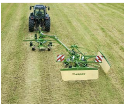
Swathing all material to the right, forming one single swath This is the swath presentation that suits high-capacity harvesters and light crops.
