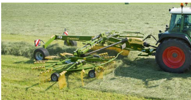
Swadro TC und TC Plus twin-rotor centre delivery rakes 5.70 m-10.00 m work widths
