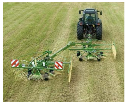
Swathing all material to the left, forming a twin swath This mode of swathing is selected to tailor swath sizes to small harvester capacities and in dense and leafy crops and for making night windrows.
