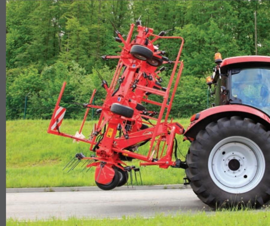
With the GF 8712 and 10812 tedders considerable working width, the small-diameter rotors limit rear overhang so that it can be used with lower power tractors. The unique folding design allows for exceptionally low transport height and convenient operation from the tractor seat.
