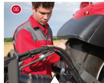
Greasing the PTO shaft.
