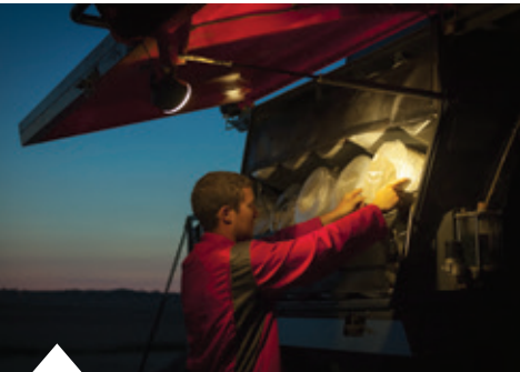
Twine box lighting allows easy night time refilling.
