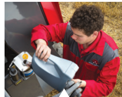
Refilling the automatic chain oiler.
