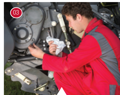
Checking the cutter gearbox oil level.
