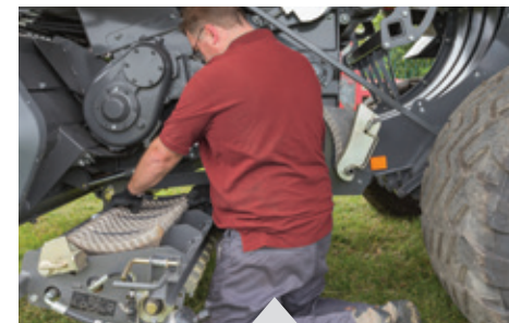
Ample accessibility offering straightforward knife removal
