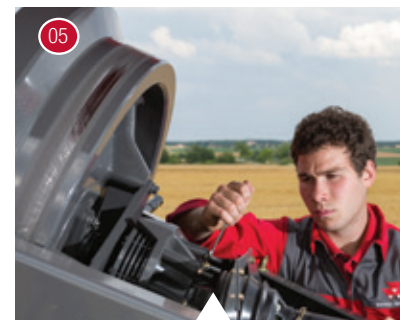
Adjusting the flywheel slip clutch.
