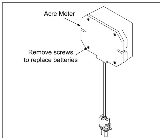
Figure 4-9: Battery Replacement
