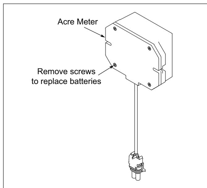
**Figure 3-16: Battery Replacement**
