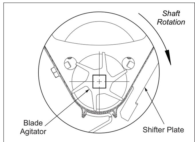
**Figure 2-5: Blade Agitator Orientation**
