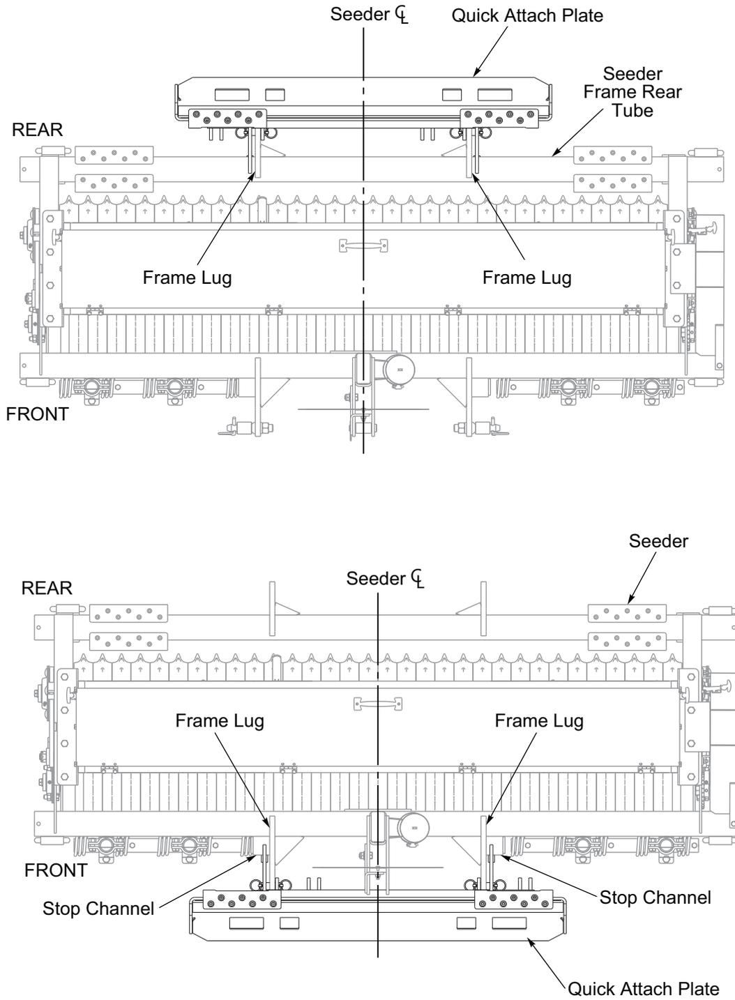
Figure 2-3: Quick Attach Plate Mounted - Centered
