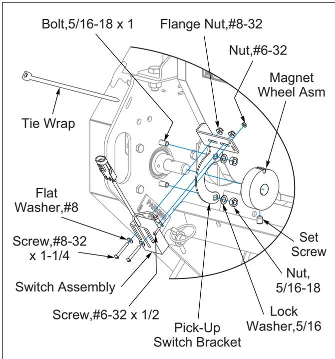
**Figure 2-11: Pick-Up Switch Bracket**
