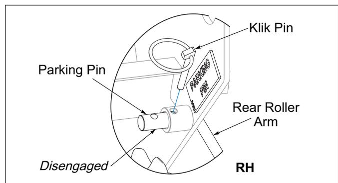
**Figure 3-1: Parking Pin Disengaged**
