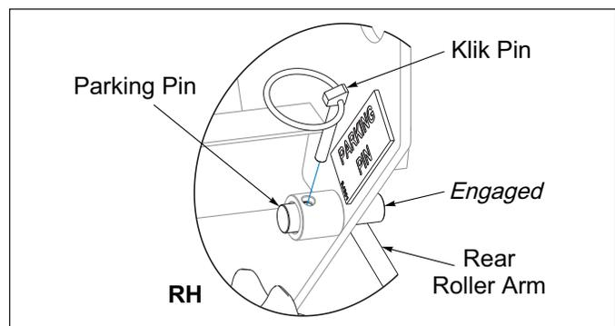
**Figure 3-2: Parking Pin Engaged**
