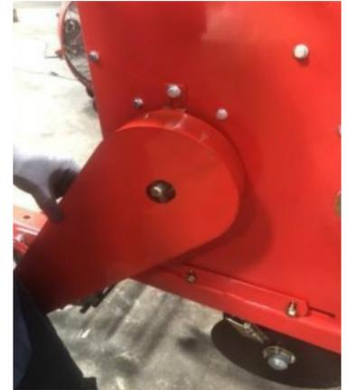
**Step 12:** Install back bracket bolt out during roller assembly.
