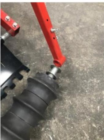
**Step 15:** Install the tension spring.
