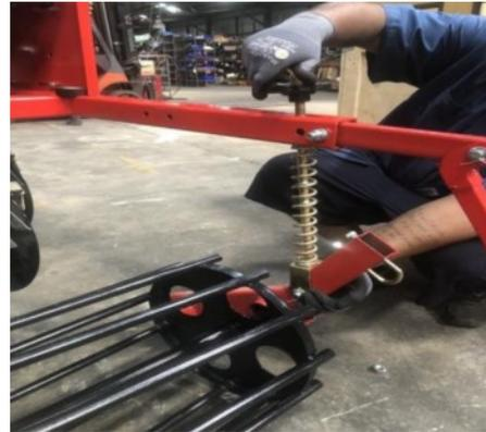
**Step 9:** Install Roller Support Plates WITH FRONT BOLTS ONLY! THE BACK BOLTS ARE INSTALLED AFTER THE CHAIN GUARDS ARE INSTALLED.
