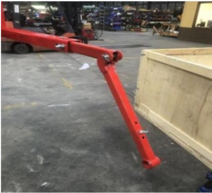
**Step 8:** Attach and install the roller adjustment rod.
