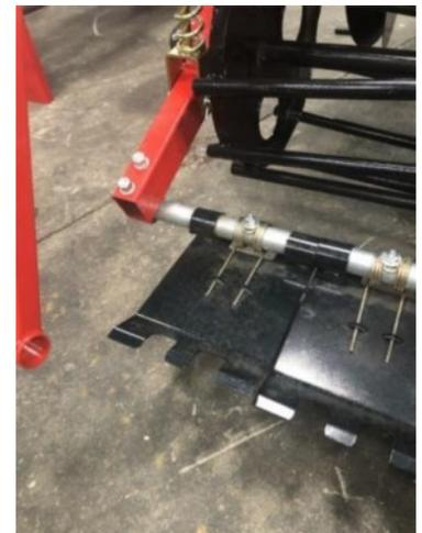
**Step 14:** Install the packer wheel assembly.
