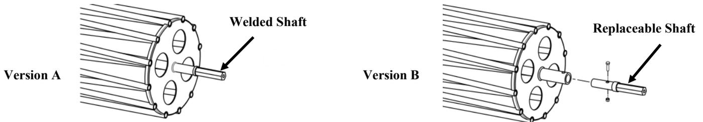
**NOTE 2:** If for any reason the roller arm needs replacing, please check the image below to determine your version, along with the serial number. These parts are not interchangeable.
