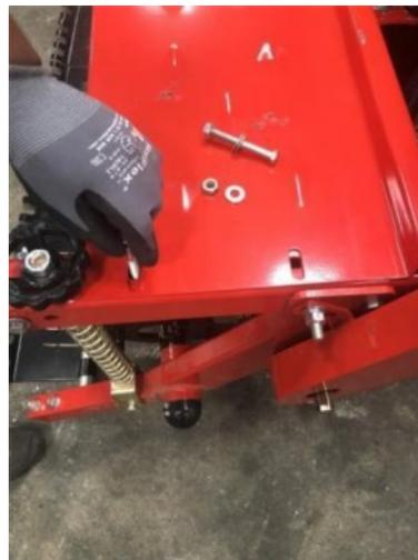
**Step 13:** Attach spring-loaded scraperboard.
