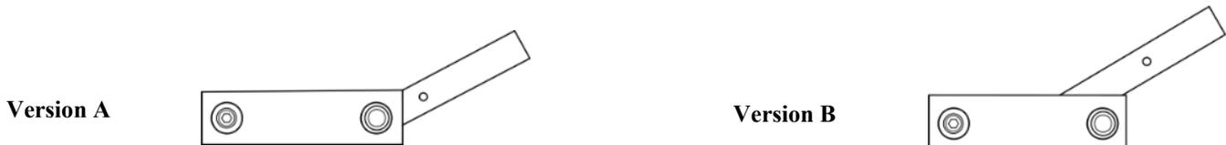
**NOTE 3:** There are two versions of the roller arm dust caps. Version A is a domed plastic cap. Version B is a low profile metal cap (Grease zerk is not required) . These parts are interchangeable.
