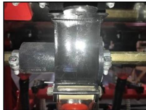
The LARGE SEED front section is usually driven with an 11-26 Gear ratio, while the back LEGUME SEED section is being reduced to put out less with a 12-40 Gear Ratio.
