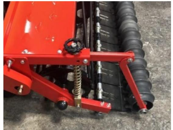
The top link on the tractor should be properly adjusted to carry the machine level in an operating position. During operation, the tractor lift must be fully lowered to allow the machine to follow the contour of the ground.
