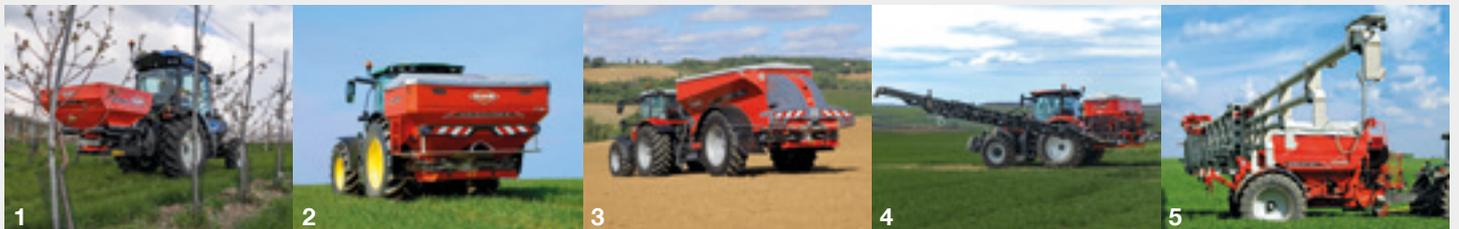
1. MDS: Mounted centrifugal fertiliser spreaders - 2. AXIS: Mounted centrifugal fertiliser spreaders - 3. AXENT: Trailed centrifugal fertiliser spreaders - 4. AERO 32.1: Mounted pneumatic fertiliser spreaders - 5. AERO GT: Trailed pneumatic fertiliser spreaders
