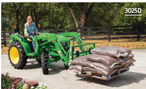
63.6 IN (161.5 CM) TURNING RADIUS. As measured from the inner rear tire with a 300E loader. To maneuver around tight spaces. Add optional pallet forks for even more versatility.
