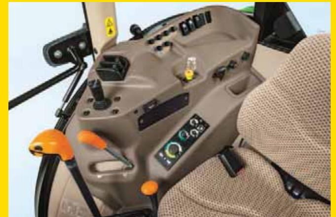
Improved ergonomics, fingertip controls and a joystick for two additional SCVs help you to work more efficiently and comfortably.
