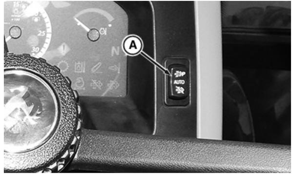
Exhaust Filter Cleaning Mode Switch—Location
