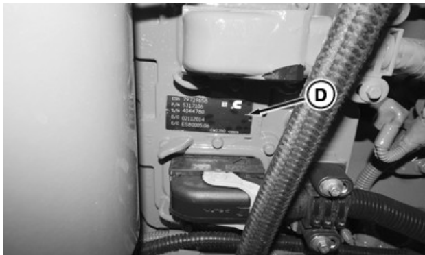
Engine Control Module (ECM) Dataplate (D) is on the Left-Hand Side of the Engine (on Front of the ECM)
