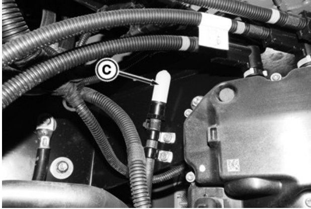
The DEF tank vent filter (C) is in the battery compartment, above the DEF dosing unit.
