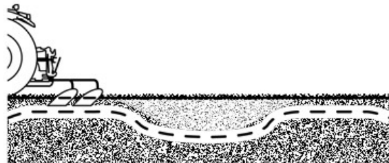
High Response Causes More Depth Variation If Soil Varies
