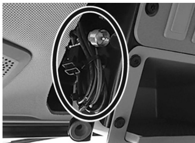
Antenna and Power Cables
