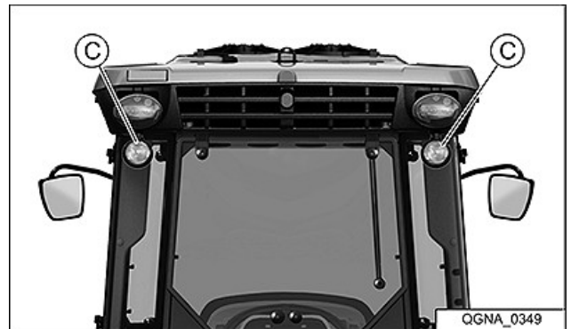
B—Light Switch C—Rear Worklights
