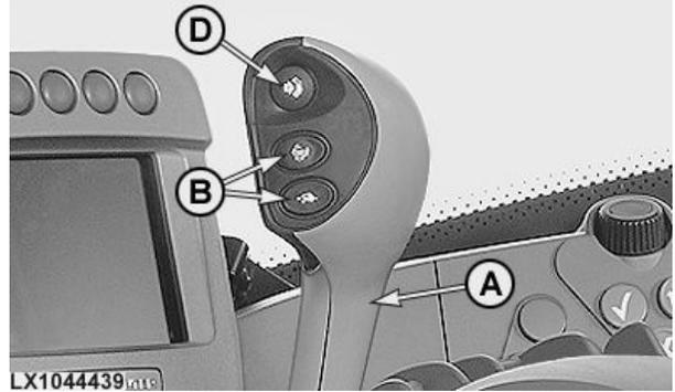
Range-shift lever and switches (with hand clutch)
