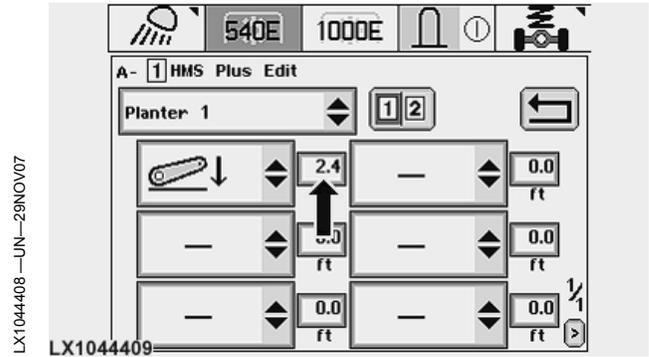
Step 2: Enter distance the tractor moves until the next function is activated
