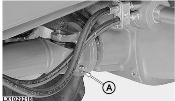
capable of running, disconnect universal-jointed drive shaft by taking out screws (A). This prevents excessive wear on the tires.
