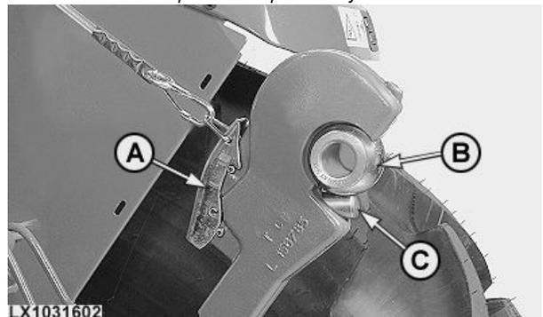
*Coupler hook operated by means of a control cable*
