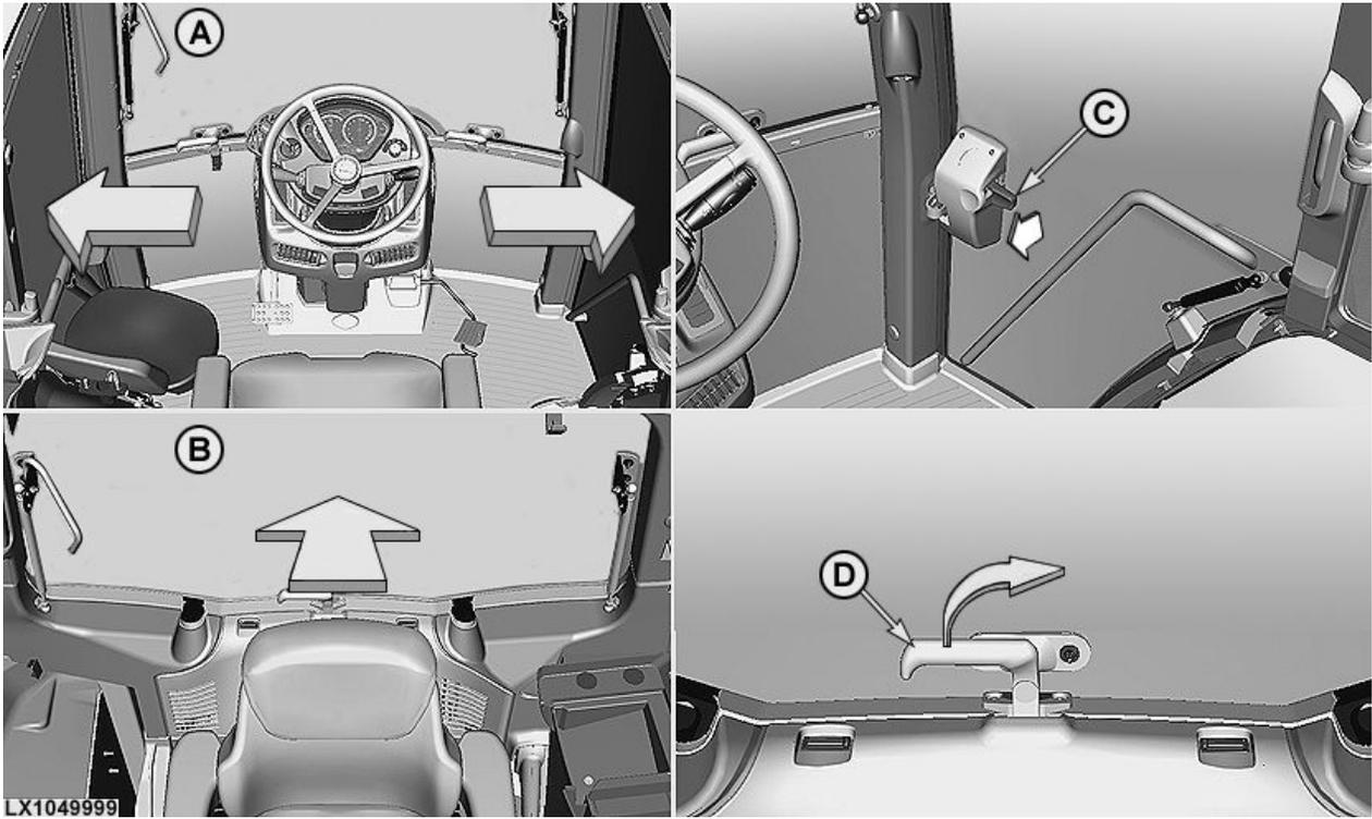
In an emergency, it is possible to exit the cab through the two doors (A). To do this, pull lever (C) to release the door and then push it open.
