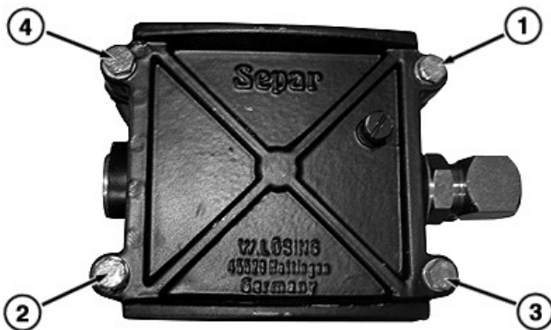
Lid Cap Screw Tightening Sequence
