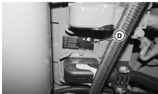
RXA0160139—UN—07JUL17 Engine Control Module (ECM) Dataplate (D) is on the Left-Hand Side of the Engine (on Front of the ECM)
