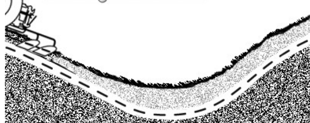
RXA0163995—UN—18JUL18 In rolling terrain, low value causes more depth variation.
