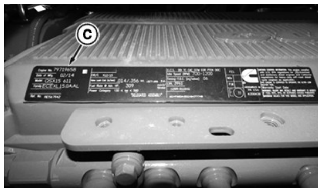
RXA0160138—UN—07JUL17 Engine Serial Number Plate (C) is on the Left-Hand Side of the Engine Valve Cover
