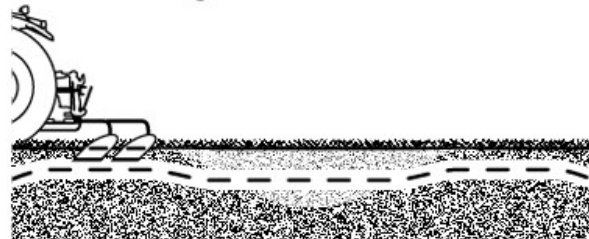
RXA0163994—UN—18JUL18 If soil varies, middle value causes less depth variation.
