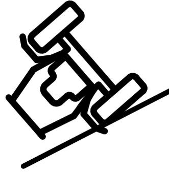
Avoid starting, stopping or turning on a slope. If the tires lose traction, disengage the PTO and proceed slowly, straight down the slope.
