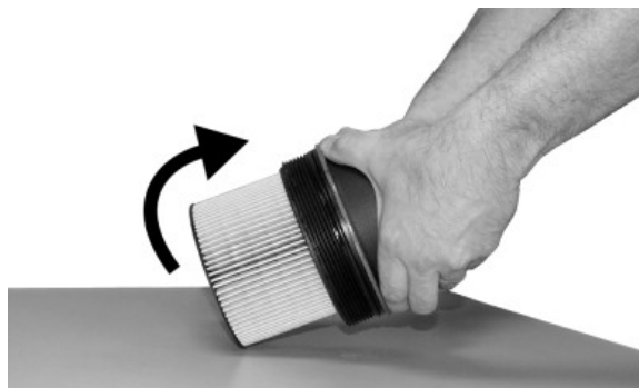
While Holding Cover, Strike Filter Against Solid Surface
