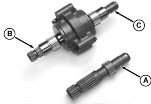
A—1000 RPM Stub Shaft C—540 RPM End B—1000 RPM End
