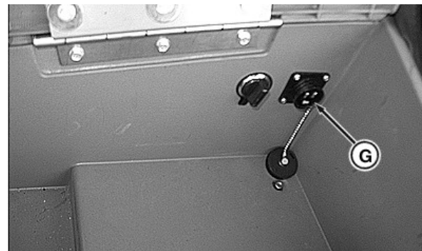
Accessory Electrical Outlet In Storage Box
