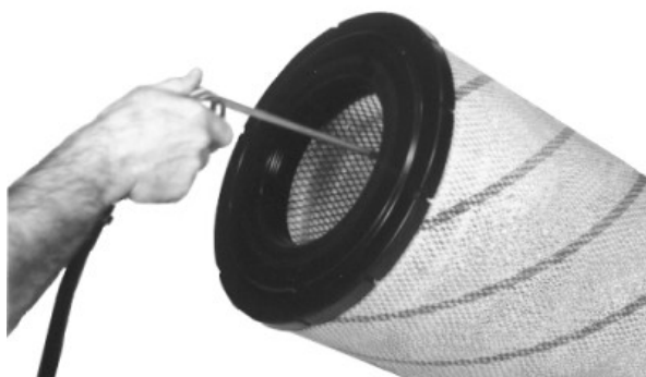
Clean And Inspect Primary Filter
