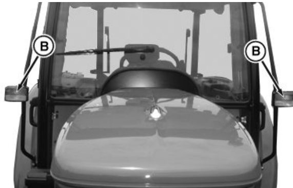
Front Turn Signal Lights
