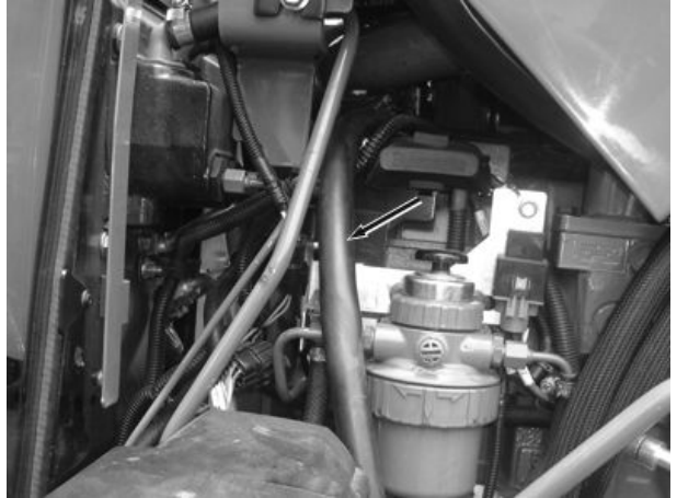
Rocker Arm Cover Ventilation
