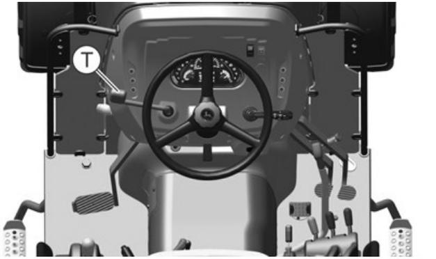
Reverse Drive Lever (mechanically actuated) (5GV, 5GN)
