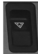
Trailing Lights Switch
