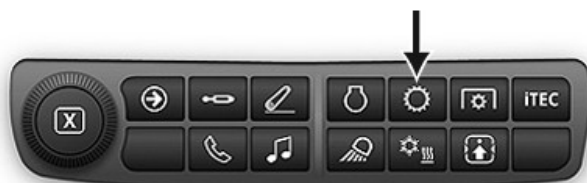
Transmission Shortcut Button on Navigation Bar
