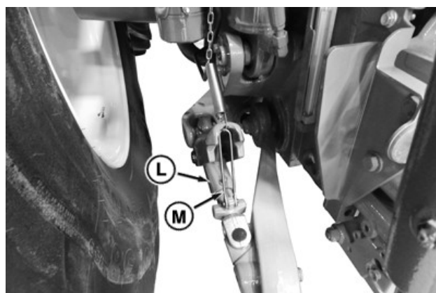
RXA0156045—UN—01DEC16 Sway Latch Lever (Left-Hand Side Shown)
