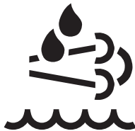
RG22487—UN—21AUG13 Diesel Exhaust Fluid Indicator
