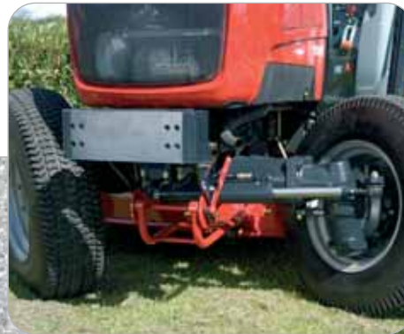
The 4-wheel drive axles maintain tight turning circles and excellent ground clearance
