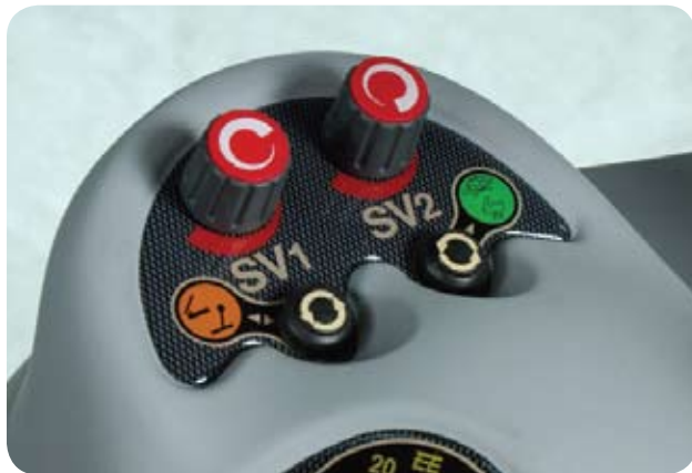
SV1/SV2 pre-set adjustment speed, Dyna-VT operating modes, and range selection are accessed in one easy-to-access location.
