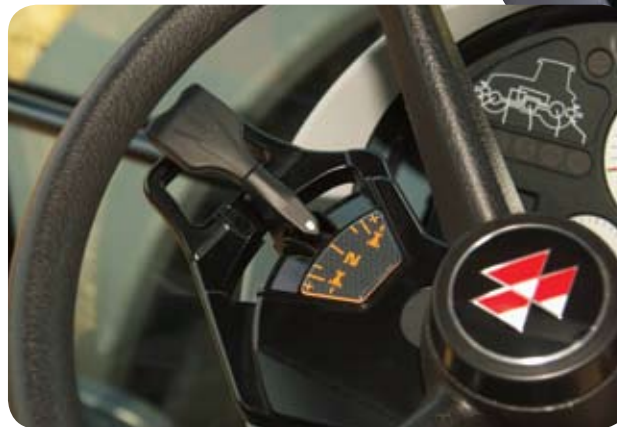
The Power Control lever offers convenient left-hand speed control.
