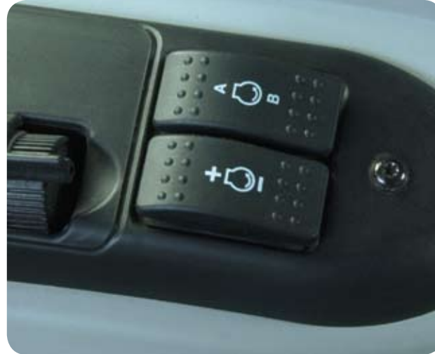
Two EEM switches located on the right hand console allow the operator to set two custom engine speeds.
