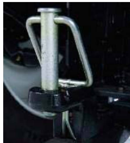
A swinging drawbar is standard equipment, and a high-capacity, heavy-duty drawbar is optional for applications where extra-heavy upward and downward loads are expected, such as with front fold planters, liquid manure wagons and large grain carts. The auto-pin hammerstrap (shown above) automatically drops and latches the pin when you hook up to implements.
