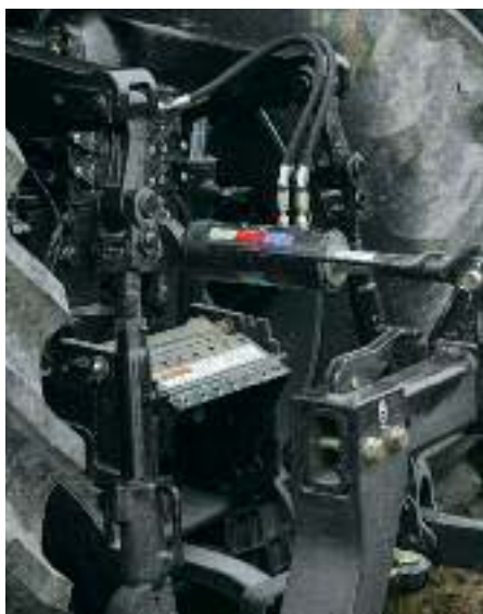
Hydraulic top link option allows for in-field adjustments and easier implement hook up.
