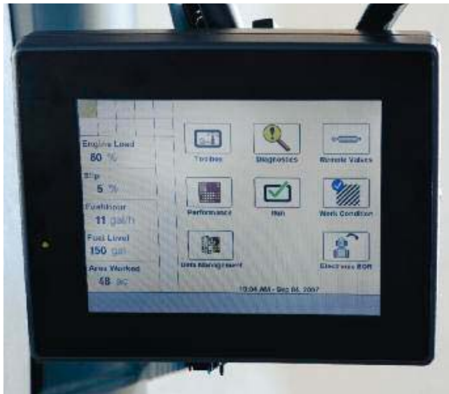
Use the IntelliView™ Plus II color monitor located on the right-hand monitor bar to: control the IntelliSteer™ auto steering system; view and change the front corner post functions; operate ISO 11783 implements of any brand.
